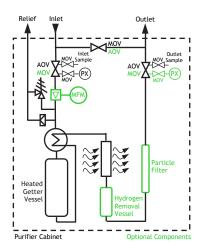
**Getter** purifiers use getter material, typically at elevated temperatures, to remove impurities that react with the getter and chemically bond to it. This chemical bond, once made survives for the life of the purifier.
