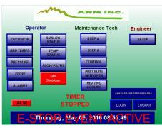
Main entry screen, with options for 3 levels of pass word protected operation.
