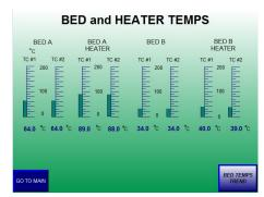
Typical indication screen, with graphic display of bed temperatures.
