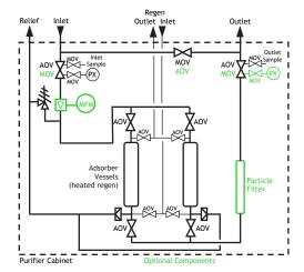
**Adsorber-Reactive Catalyst** purifiers use adsorber material, or in certain instances a reactive catalyst, to remove impurities from a wide variety of gases.
