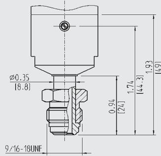
1/4" T-Connector, Weld Stub
