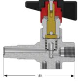
\* HRGADSVL-E: diaphragm shut-off valve long extantion
