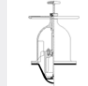
Non-Rising Handwheel with indicator Valves sizes: DN200 to DN350 (8" to 14")
