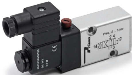
Solenoid valve , attached to the actuator to create an electro pneumatically actuated ball valve. DC 24V, 2.5W 4/2 Way for double acting and spring return. Enclosure IP65 Option for: 110VAC, 50HZ. Option for: 3/2, 5/2 Way.
