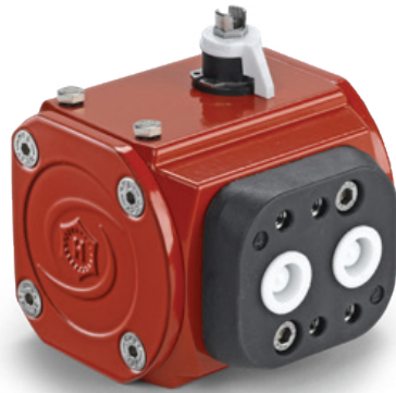
Standard 90 degrees. Aluminum pneumatic actuator , Operating Pressure: max. 8 bar (116 PSI). Standard working temperature -32°C to 90°C (-25.6°F to 194°F)
