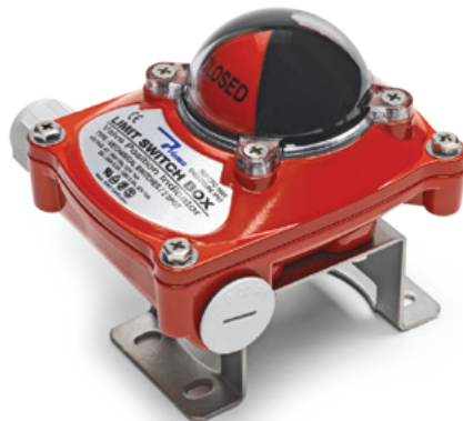
Electro Mechanical limit switch for visual and electric indication of actuator position. Enclosure IP67, voltage: AC: 250V 16A, 125V 16A DC: 250V 0.3A, 125V 0.6A, 30V 10V
