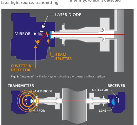
Fig. 2: The Laser 3 Plus installed across a stack, with line lock system (circled)
