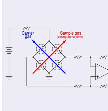
The Thermal Conductivity sensor
