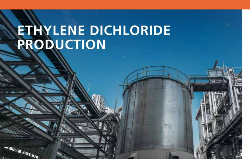
The predominant global method for PVC production is the ethylene-based route, using ethylene dichloride (EDC) as an intermediate. EDC production requires gas analysis at several points, for process control and quality monitoring. A variety of technologies are needed to measure the range of gas components within the process.
